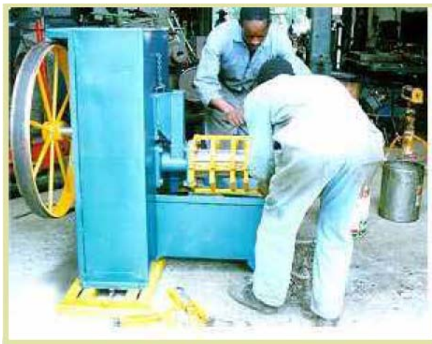
JCL Oil Press based on Sundhara design JCL Oil Press installed at Makosa in 1999 by BUN ( Photo BUN 99 )
