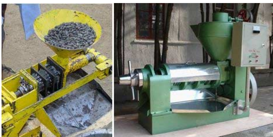
Figure 15. Examples of a Bielenberg Ram Press and a commercially available pressing system for J. curcas seeds.
