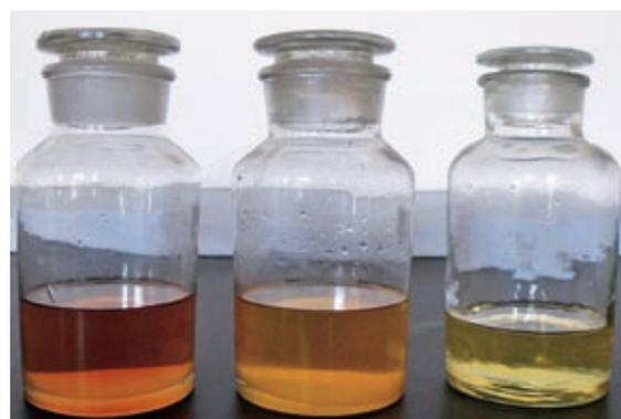
Crude *Jatropha* oil from XTBG and biodiesel produced: left, *Jatropha* oil; middle, Biodiesel with sulfuric acid; right, Biodiesel two-step process
