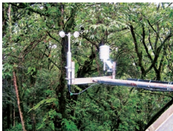
Seven-level wind speed, temperature and humid microclimate vertical observatory system and 6-level pole PAR observatory system
